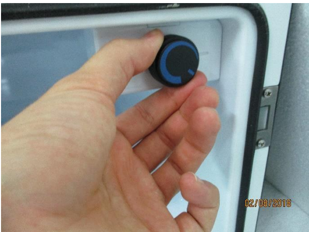
3. Remove the thermostat's knob
