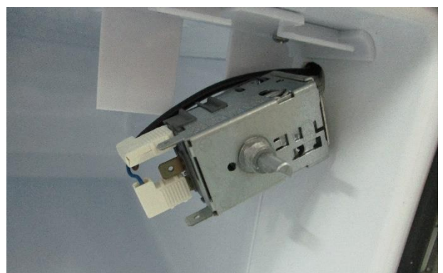
6. Disconnect the wires from the thermostat and pull it to remove the thermostat's bulb; reverse the procedure to replace the thermostat
