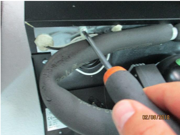
1. Unscrew the bolt fixing the thermostat's bulb
