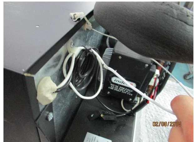
2. Remove the thermostat's bulb
