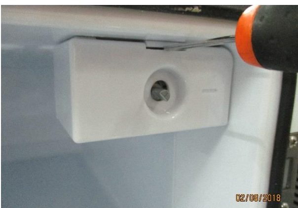
5. Use a screwdriver as a lever to remove the thermostat's box (or unscrew the 2 bolts that fix the box; depending on the model of box)
