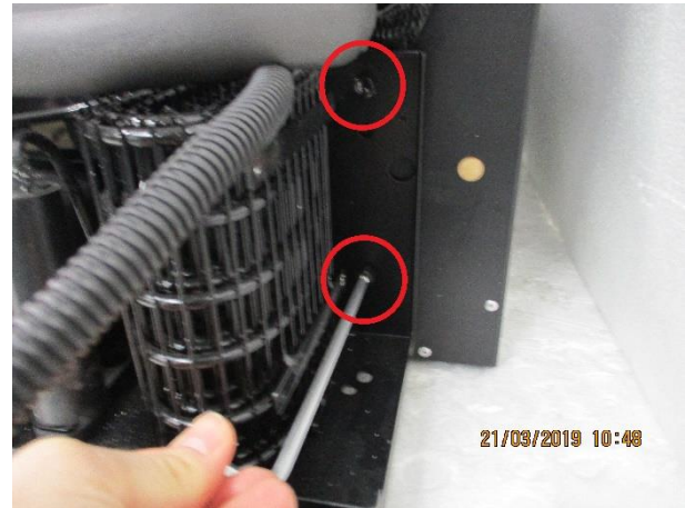
3. Unscrew the basement of the refrigerating unit (4 screws)
