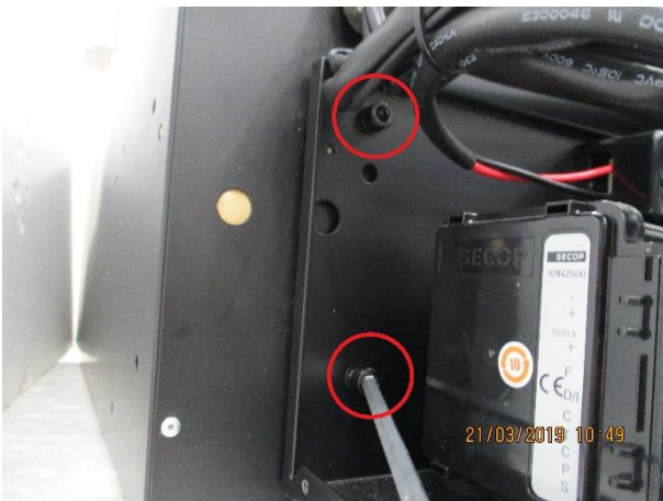
3. Unscrew the basement of the refrigerating unit (4 screws)
