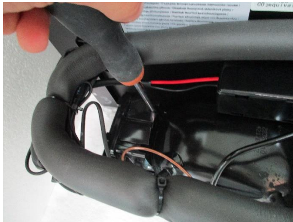
3. Unscrew the last bolt, disconnect all the wires from the ECU and remove it. Reverse the procedure to replace the ECU
