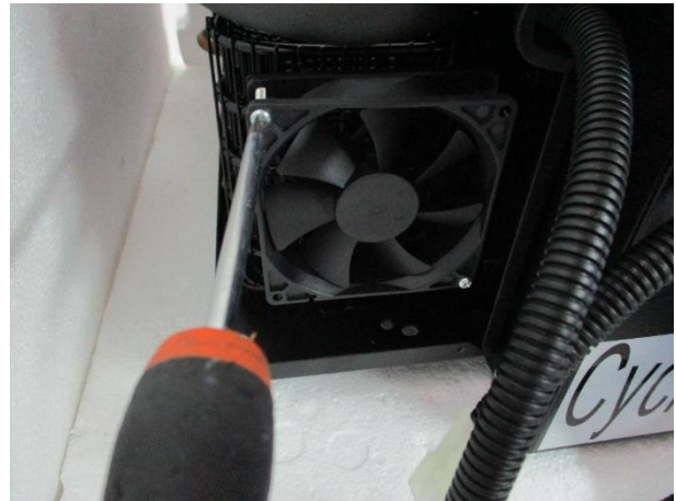
2. Unscrew the 2 bolts fixing the fan and reverse the procedure replacing the fan with a new one
