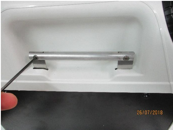
1. Unscrew the 2 handles (4 bolts)
