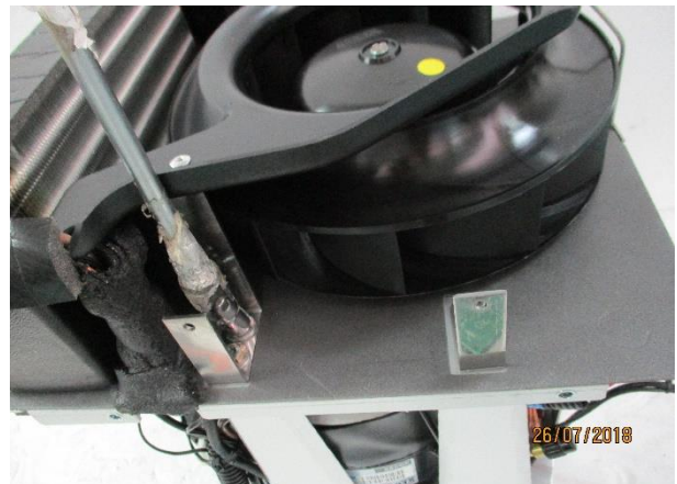
6. Unscrew the 4 brackets (8 bolts)
