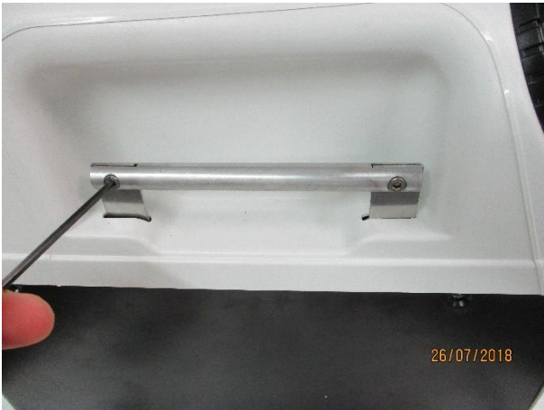
1. Unscrew the 2 handles (4 bolts)
