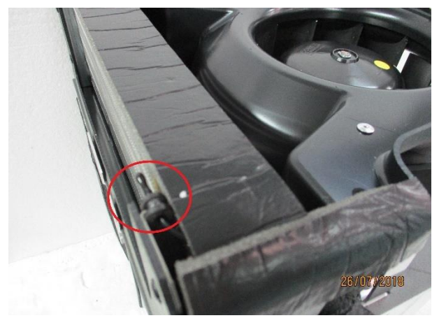
6. Remove the probe reverse the procedure to replace it
