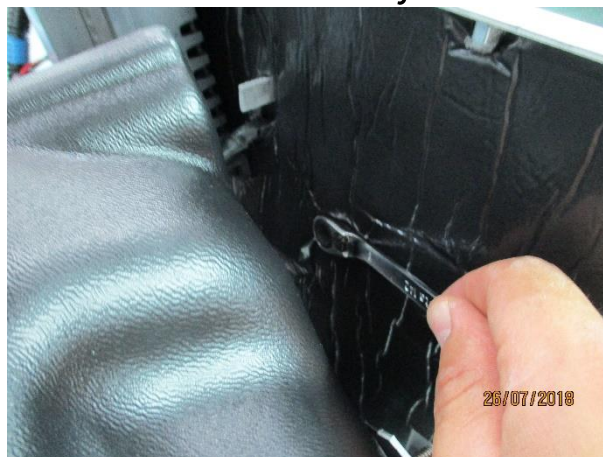
11. Unscrew the 3 bolts fixing the blower, disconnect the blower's wires from the ECU, and reverse the procedure to replace it
