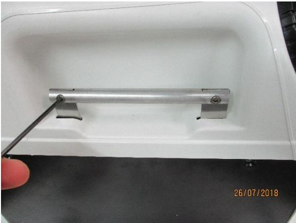
1. Unscrew the 2 handles (4 bolts)
