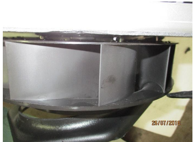
10. Watch from the upper side to see the location of the 3 bolts (one screw is behind the ECU so you need to rotate it)
