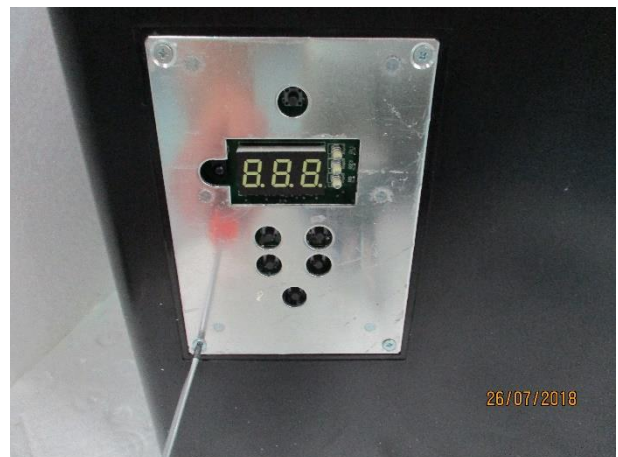
4. Unscrew the display (4 bolts) and disconnect the 2 wires connected
