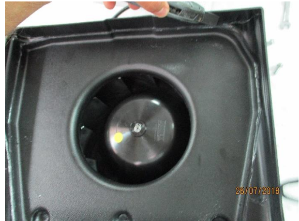
8. Use a cutter to remove the gasket and remove the fan
