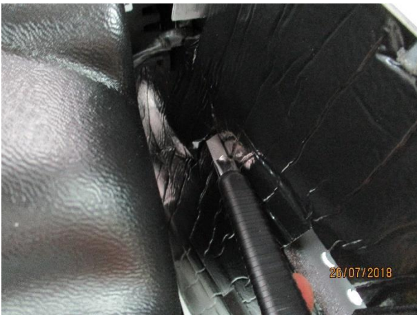
9. Cut the protection sponge near the 3 bolts fixing the evaporator fan
