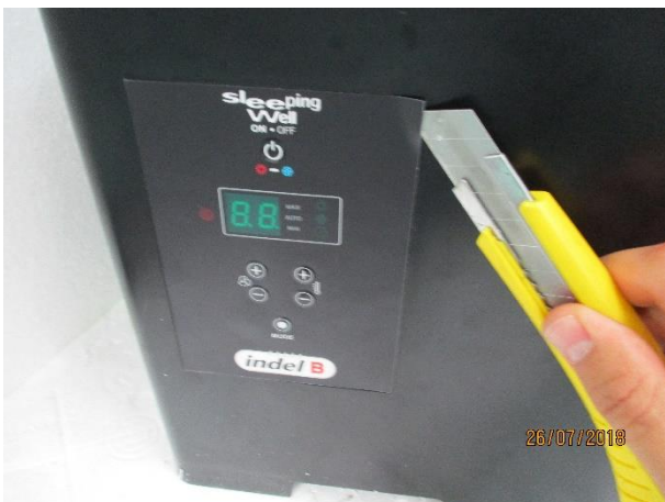
3. Use a cutter to remove the display's label
