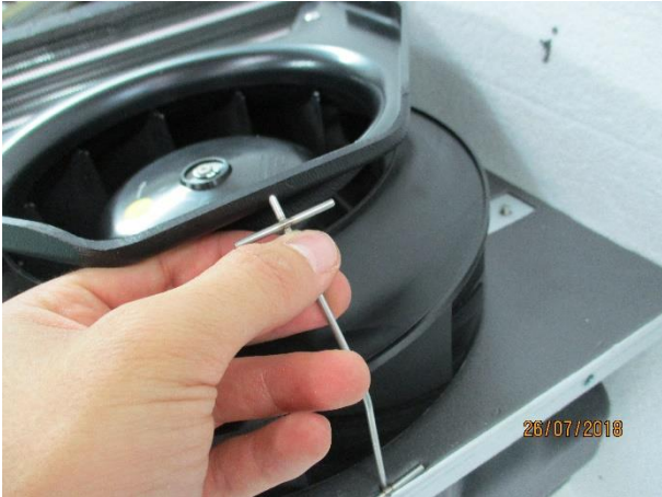
7. Remove the pin holding the evaporator fan
