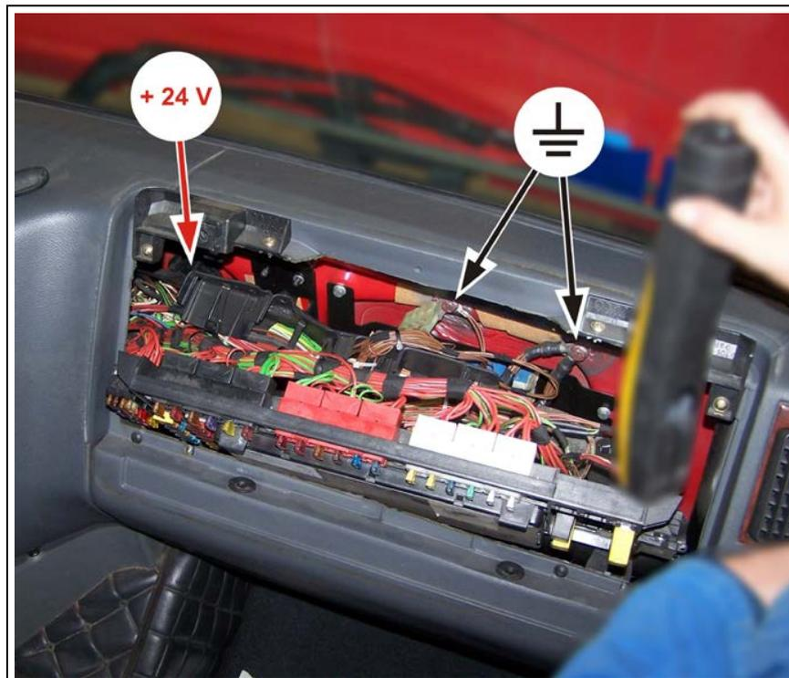
Method for connection **directly to the vehicle's battery**:
