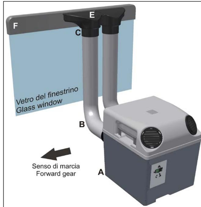
**WARNING:** when driving it is necessary that **visibility of the rear-view mirrors and through the side windows is NOT compromised**. To this end, endeavour to place tubing, snorkel and gaskets in the least obtrusive manner possible; if visibility is compromised **reposition “CUBE”** and its relative components in a suitable place.
