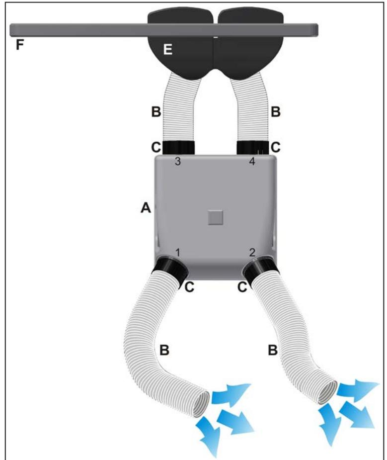
**HOT MODE:** connect 1 piece of flexible tubing (B) between one air output nozzle (1 or 2) and opening 3; the unused air output nozzle (1 or 2) must be sealed with the supplied lid (D) placed in the opening (C). Warm air will exit from opening 4.
