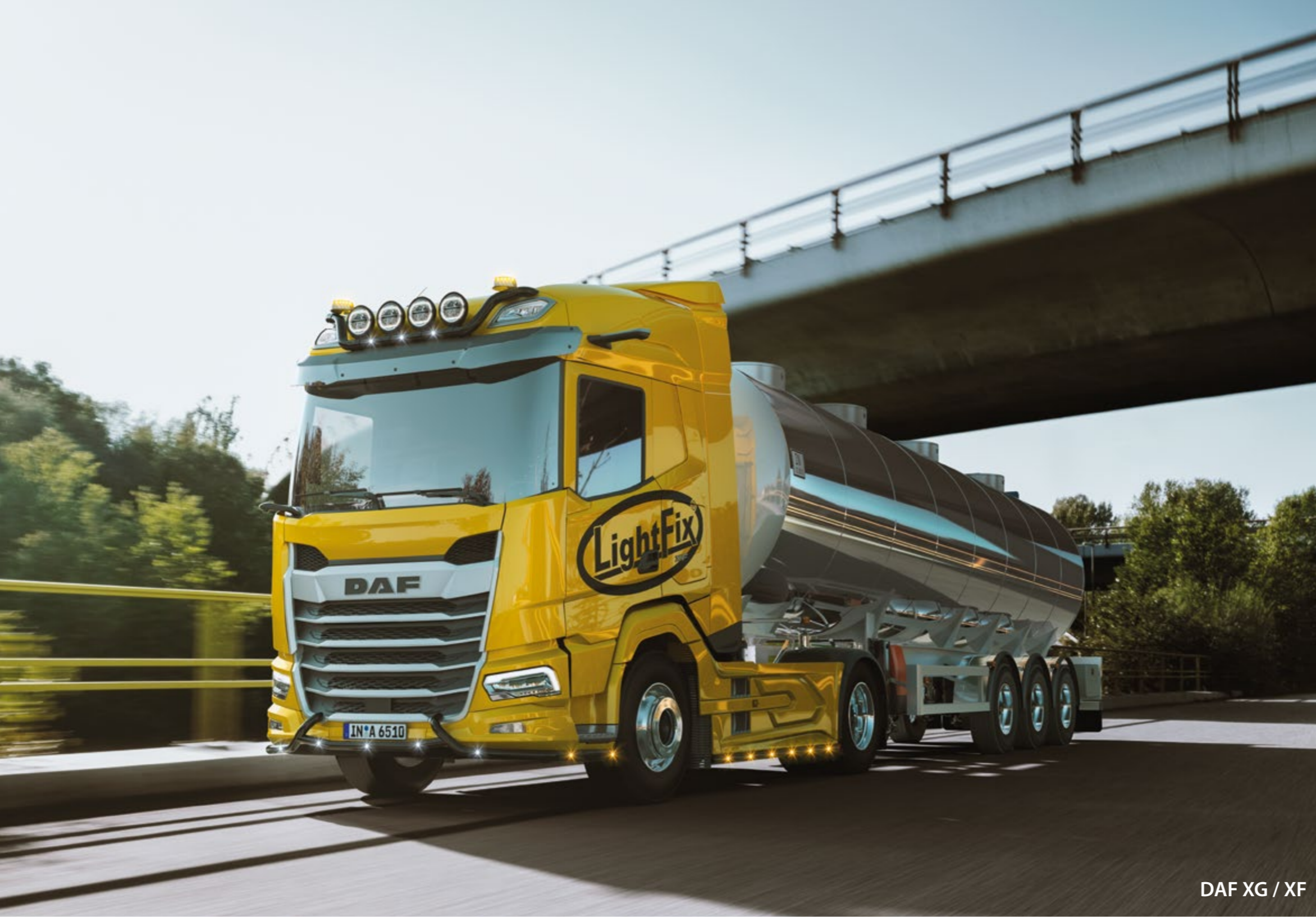
28705-9-B - LightFix - SKY-LIGHT "H-MAX" Lightbar for mounting a maximum of 4 spotlights and 2 beacons stainless steel - black powdercoated - Ø 70mm - prewired incl. amber LED on the side and red LED in the tube ends
