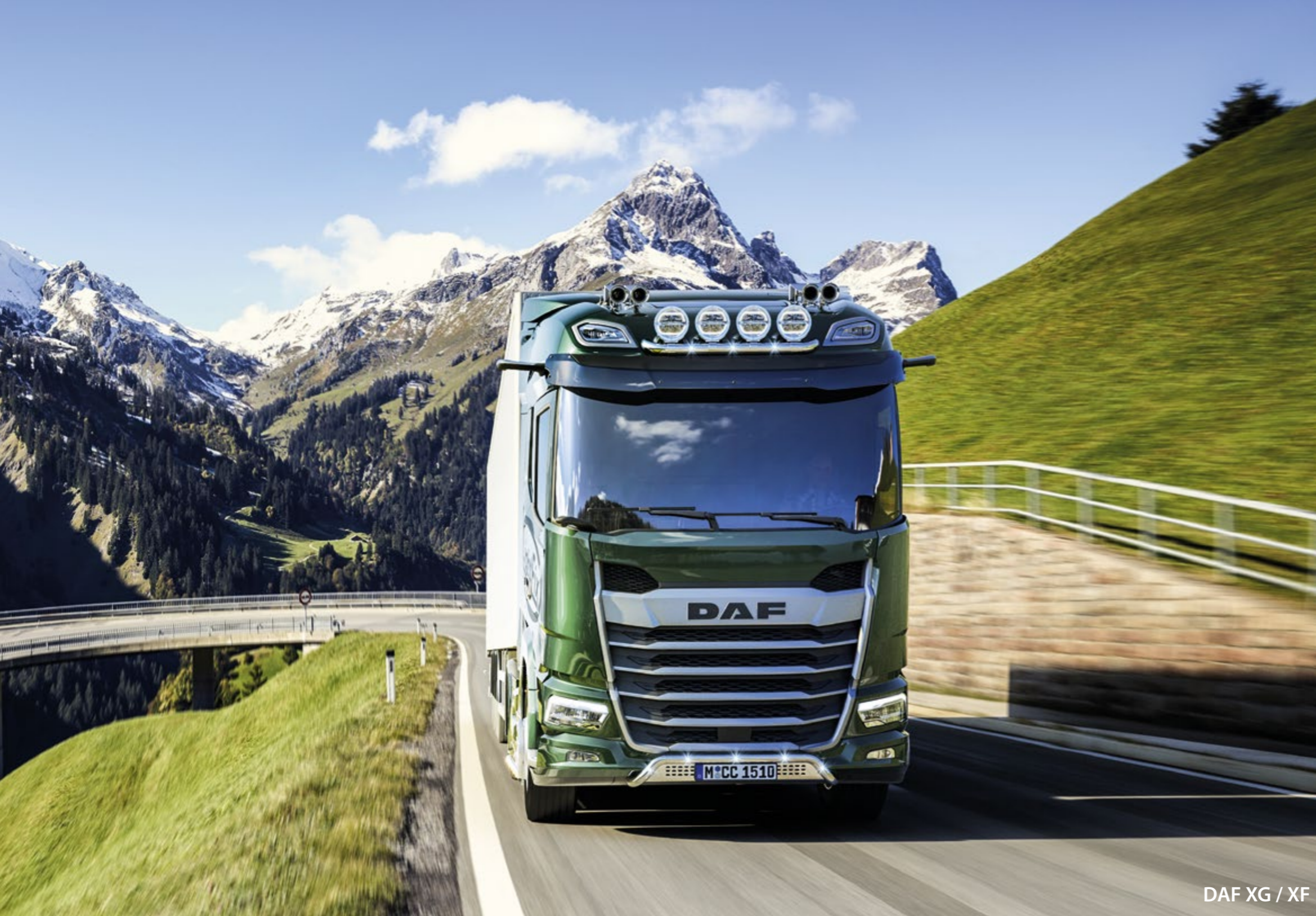
28705-9-P - LightFix - SKY-LIGHT "H-MAX" Lightbar for mounting a maximum of 4 spotlights and 2 beacons stainless steel - polished - Ø 70mm - prewired incl. amber LED on the side and red LED in the tube ends
