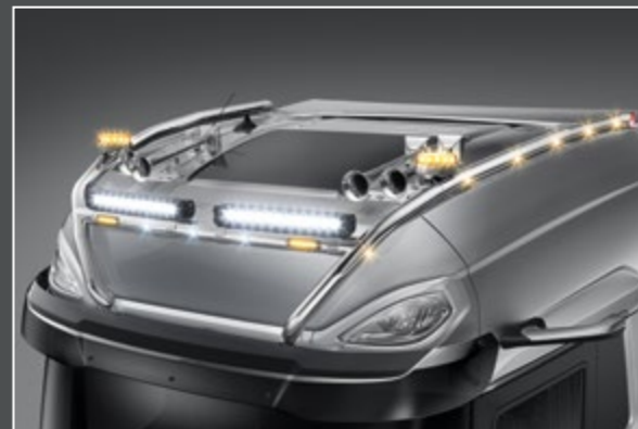
28706-9-P - LightFix - SKY-LIGHT "H-MAX" Lightbar for mounting a maximum of 6 spotlights and 2 beacons stainless steel - polished - Ø 70mm - prewired incl. amber LED on the side and red LED in the tube ends
