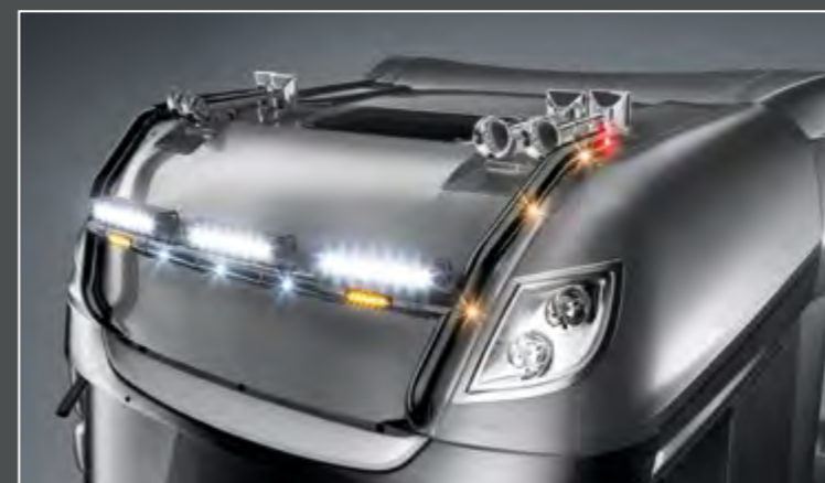
28701-6-B - LightFix - SKY-LIGHT "H-TYPE" Lightbar for mounting a maximum of 6 spotlights and 2 beacons stainless steel - black powdercoated - Ø 70mm - prewired incl. red LED in the tube ends
