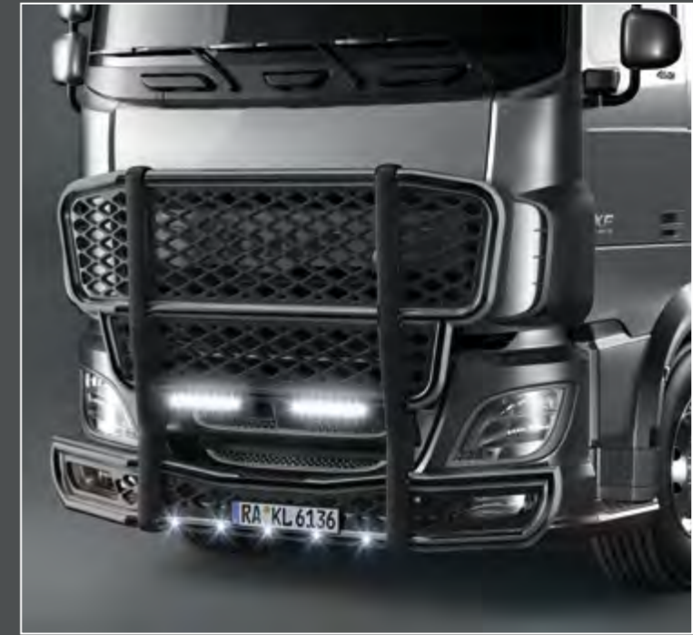
28760-2-B - LightFix - FRONT-PROTECT "BIG NORDIC" Stainless steel front protection bar incl. black net made of ABS black powdercoated - Ø 70mm - prewired
