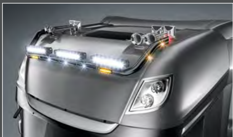
28701-4-B - LightFix - SKY-LIGHT "WILDLIFE" Lightbar for mounting a maximum of 6 spotlights and 2 beacons stainless steel - black powdercoated - Ø 70mm - prewired incl. red LED in the tube ends
