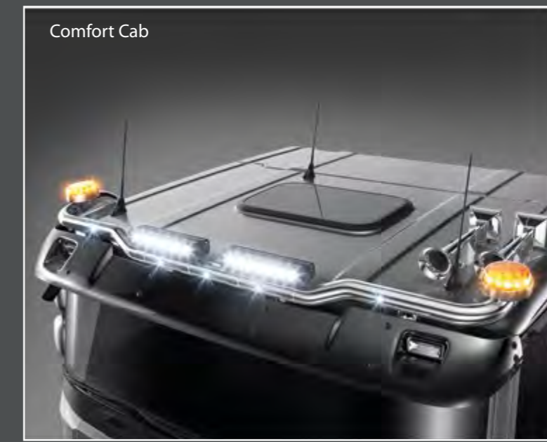
28702-2-P - LightFix - SKY-LIGHT Lightbar for mounting a maximum of 4 spotlights and 2 beacons stainless steel - polished - Ø 70mm - prewired
