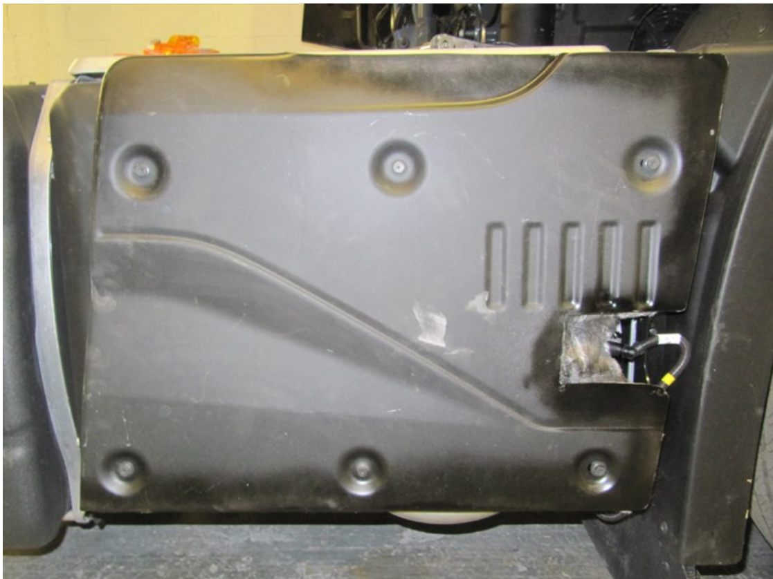
After cutting, de-burr all edges and treat with rust protector.
