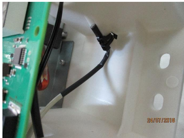
3. Remove the tilt sensor and reverse the procedure to install a new one
