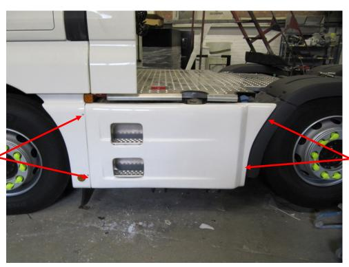
Bolt through mudwing and sideskirt return using M8x35 Screws, washers & Nyloc Nuts
