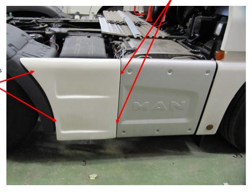
Bolt through mudwing and sideskirt using M8 Button Head Screws, washers & Nyloc Nuts.
