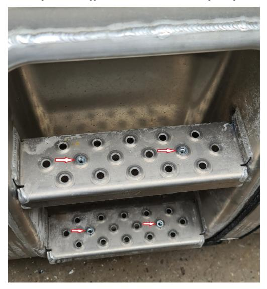
Step 2 – Fix both supplied "Aluminium steps" to the supplied fibreglass N/S Side-Skirt using:
