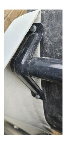
Step 5 - Remove the factory fitted bots from the middle plastic mud wing. Place the supplied fibreglass Side-Skirt between factory bracket and the factory plastic mud wing. Fit back the factory fitted bolts.
