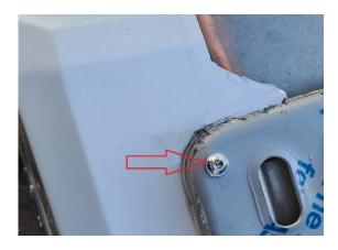
Step 5 – Kuda UK platform variant – Fit the supplied O/S Top Bracket into the top rear fixing from the tank using the supplied:
