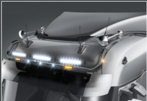
TLG20701-3-B - LightFix - SKY-LIGHT "U" Lightbar for mounting a maximum of 6 spotlights and 2 beacons stainless steel - black powdercoated - Ø 70mm - prewired
