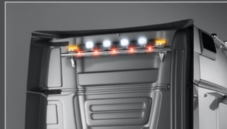
25715-3-P /-B - LightFix - REAR-LIGHT Stream Space 2500 - Big Space - Giga Space Lightbar for mounting a maximum of 4 worklamps and beacons stainless steel - polished or black powdercoated - Ø 70mm - prewired
