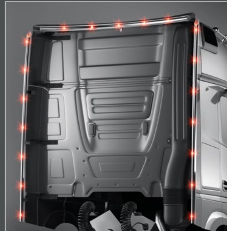
25749-1-P /-B - LightFix - ROOF-LINER - Actros Giga Space 25749-2-P /-B - LightFix - ROOF-LINER - Actros Big Space Stainless steel LED-lightbar for max. 4 work lamps and 2 beacons on the roof spoiler polished or black powdercoated - Ø 70mm - prewired Full LED-set included
