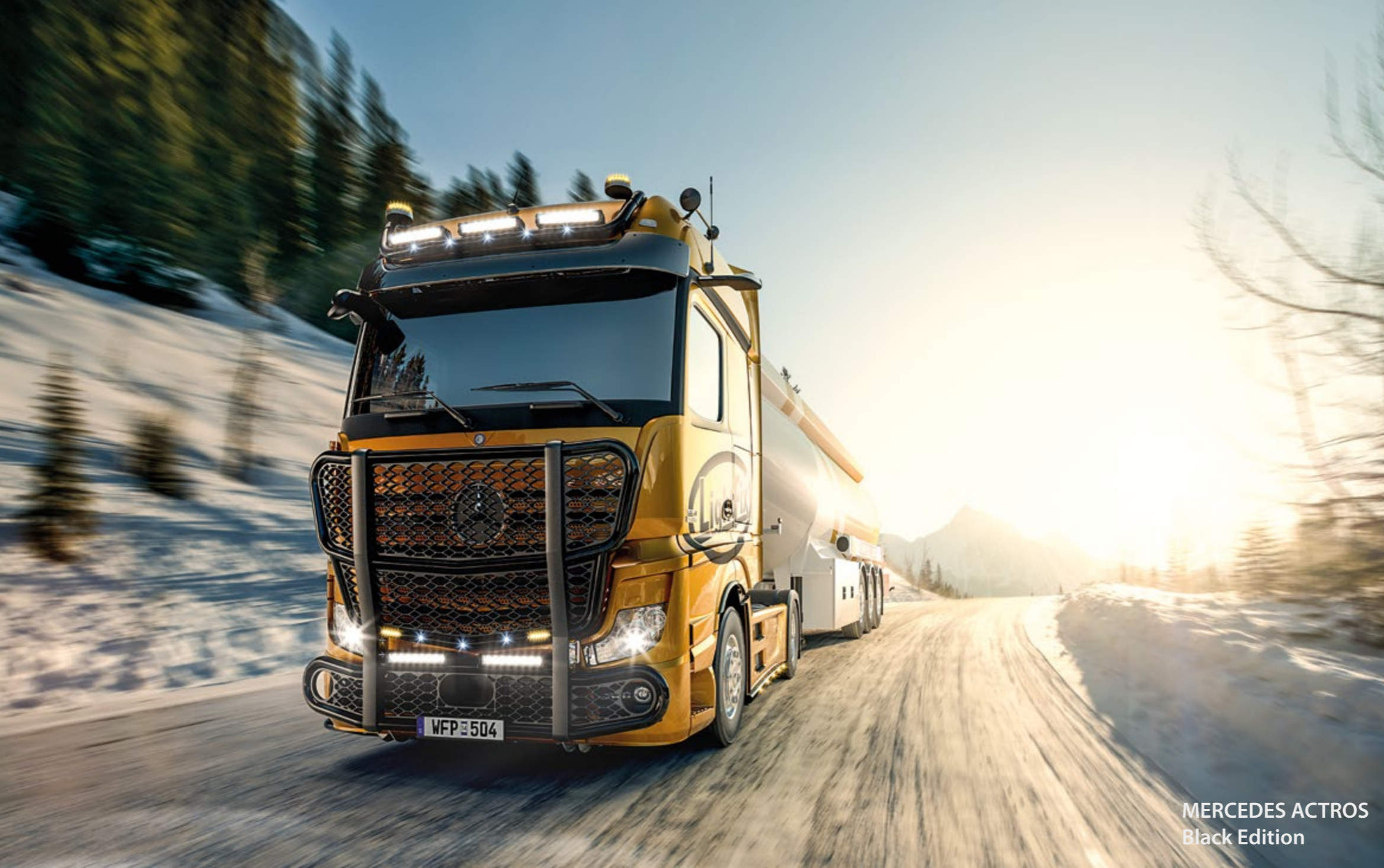
25760-2-B - LightFix - FRONT-PROTECT "BIG NORDIC" Actros 2500 mm Stainless steel front protection bar incl. black net made of ABS black powdercoated - Ø 70mm - prewired 29708-1-B - LightFix - LAZER-BRIDGE for Lazer Triple-R 1000
