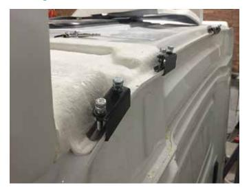
Attach gutter clamps and channel to the rear cab gutters as shown. Repeat steps 2 through 5 for the other ear.
