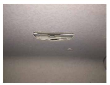
Remove both interior lights from roof lining to expose under side of cab roof. Push any wires towards the centre of the cab.
