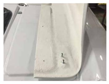
Position ear on roof using the moulded shape of the base to align correctly. Drill through the 2 pre-drilled holes into the cab roof.
