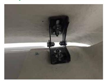
Secure front hinging brackets to spoiler blade (do not over tighten). Then lift blade up to the roof and position and secure hinges to the pre-moulded studs in the ears.
