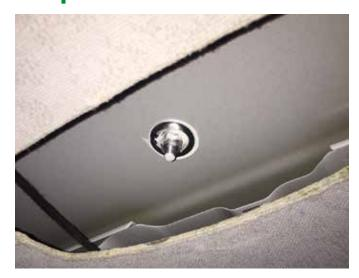
Insert 1 x M8 x 25mm Bolt through the larger of the 2 holes. Secure with washer and nylock. Insert quick screw in the smaller hole at the front of the ear.
