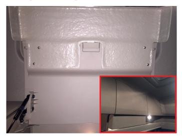
If you have the optional Topline Fascia panel supplied this is secured to the centre locker door using the supplied screws via the pre-drilled holes as shown.
