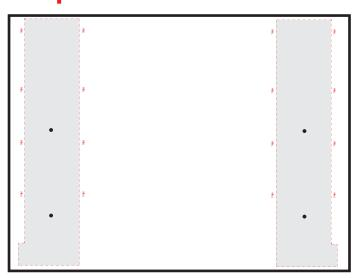
Place supplied drilling jig on locker floor. You will need to trim the jig along the marked cut lines, this will ensure that the marked holes are in the correct location. Drill holes as marked using 6mm drill bit.
