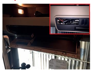
Remove N/S Small Locker by removing 4 small screws along front edge. Also remove O/S left hand small storage hole. This just pulls out.
