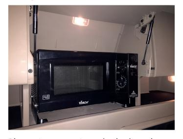
Plug microwave into the locker plug then position microwave in locker with the holes in the bottom of the legs over the ones in the locker floor drilled earlier. Drop through long bolts supplied and fasten with supplied nylocks and washers.
