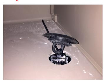
Remove rubber bung and pull through microwave preparation wire (factory fitted).
