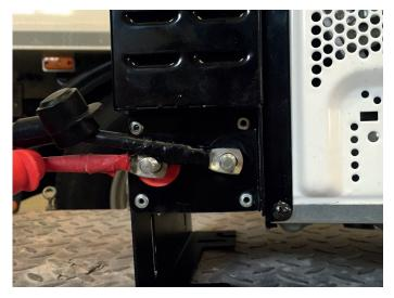
Connect small (Scania GB) supplied loom to the back of the microwave unit.
