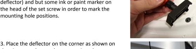
the picture and press the part against the corner of the vehicle. The correct position of the part is shown on the picture (20-25mm from the vertical edge on the side and on the middle of the styling groove.
