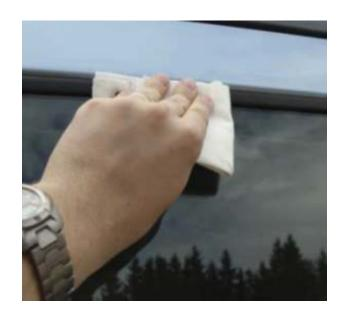
4. Mount the deflector on the door. Roll/press the deflector against the door for several minutes in order to attach the full are of the tape.
