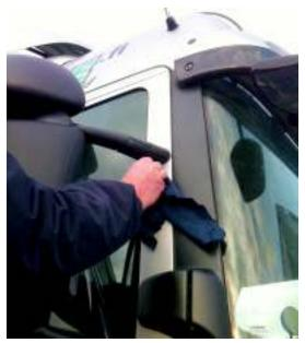
4. Mount the deflector on the door. Roll/press the deflector against the door for several minutes in order to attach the full area of the tape.
