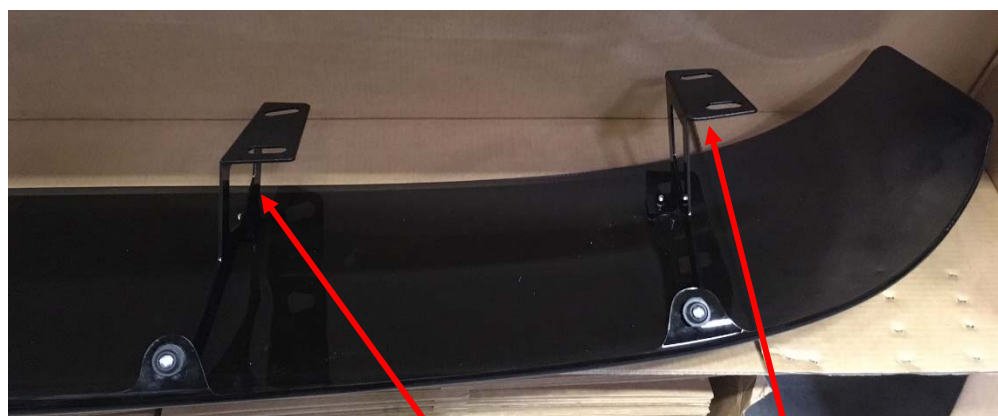
Brackets on right side of the visor. Bracket middle right (#3) Bracket right (#5)
