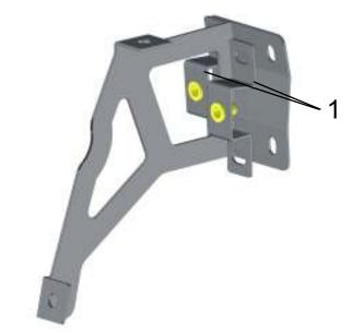
Glide the light bracket in the center brackets and mount it with M6x20mm hex screws and 6x22mm washer, but do not fully tighten yet.
