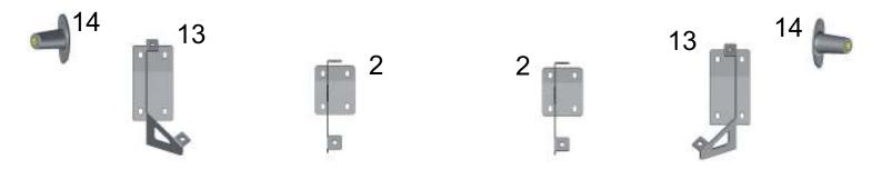
Mount the acrylic part on brackets as shown on the drawing: When you mount the side bracket you do not use parts 9 and 10.
