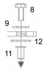
But Sikaflexon the topside of the acrylicpart which touches the cabin. Mount the acrylicpart on the brackets and tighten all screws.
