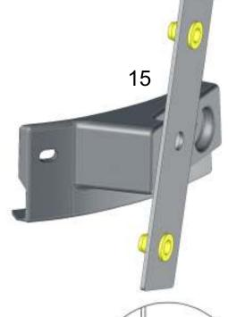
Place the visor on the vehicles roof and mark the hole positions. Drill the holes with 4,50mm bit. Now drill the holes for the center breakets for rivet nuts to size of 11,0mm with a step drill tool. Please note that the hole must be tight for rivet nut.
