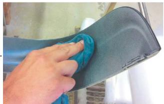
4. Remove the protection foil of the sun visors VHB-tape and carefully mount the original top part on the sun visor. Make sure you support the backside of the visor with your hand when you push the top part on the visor.
