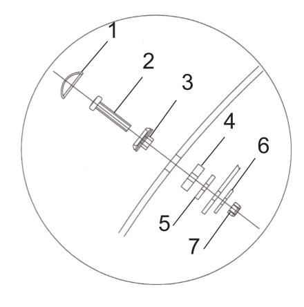
After you have mounted the acrylic part on the truck, press the marker lights (and truck lights if model 5049A) on the acrylic part. To ensure the marker light is correctly mounted on the acrylic part, check that the mounting clamps of the marker light are locked, if not open the clamps with screw driver as shown on the drawing.
