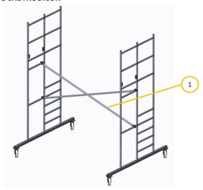
1. Click both diagonals (blue claw blocks) to the base frames (opening of the claws facing the floor).
