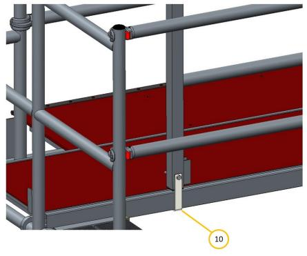
10. Put the connector around the platform profile and firmly fix the butterfly nut.
