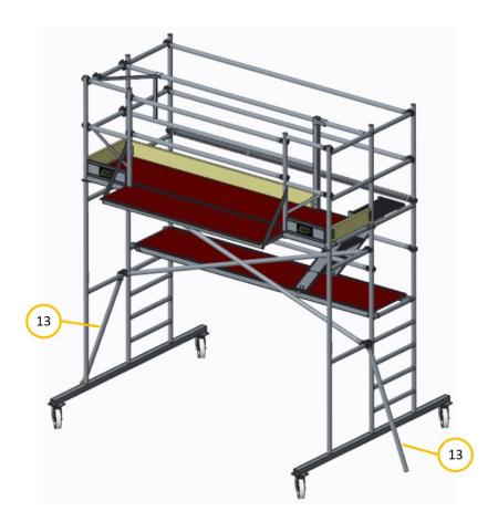
13. Attach the 2 support braces (firmly push the brace to the floor so that you get some pressure on it and it does no longer slide over the floor surface).
