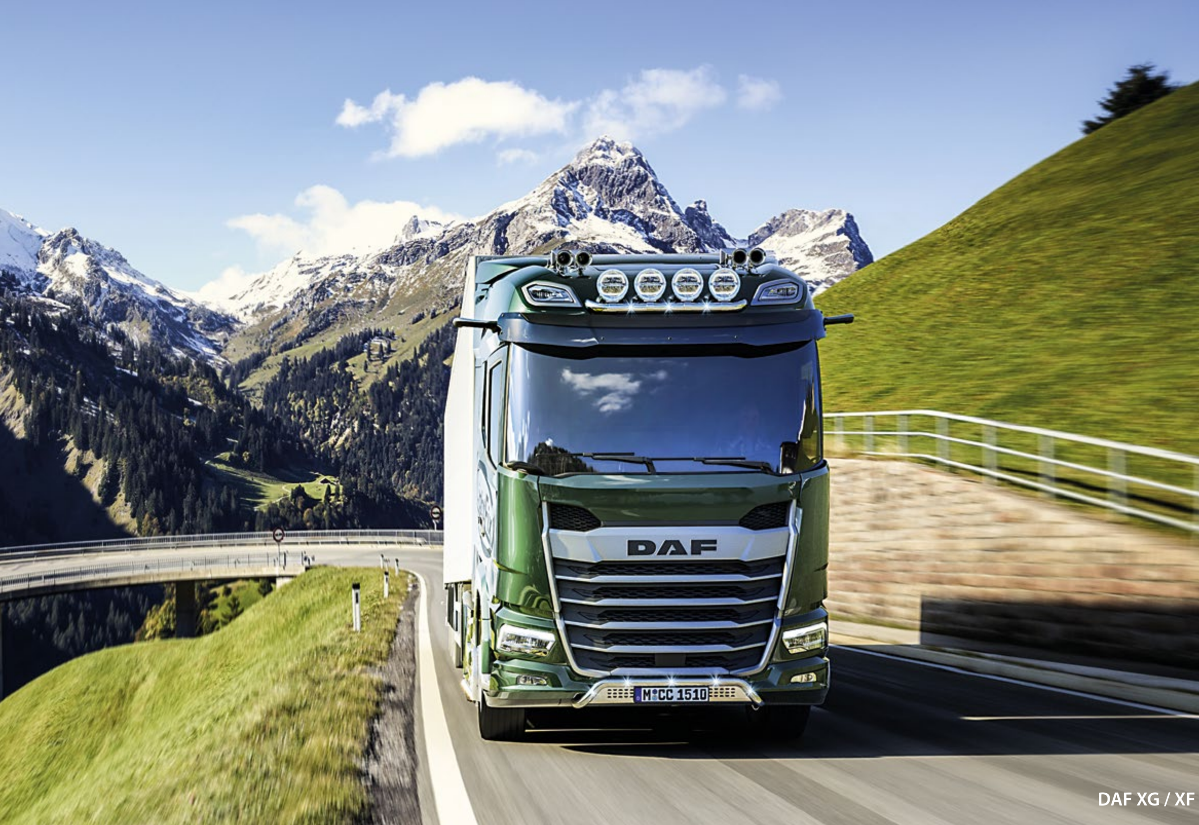
28705-9-P - 28705-12-P - LightFix - SKY-LIGHT "H-MAX" DAF XG (28705-9-P) / DAF XF (28705-12-P) Lightbar for mounting a maximum of 4 spotlights and 2 beacons stainless steel - polished - Ø 70mm - prewired incl. 8 amber LED on the side and red LED in the tube ends
