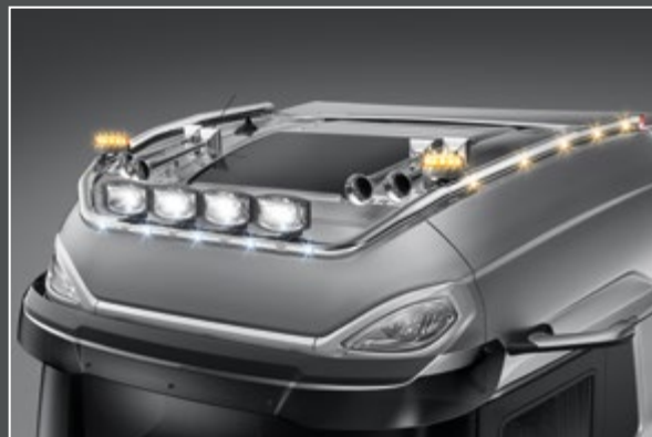
28706-5-P - LightFix - SKY-LIGHT "CLASSIC-MAX" Lightbar for mounting a maximum of 4 spotlights and 2 beacons stainless steel - polished - Ø 70mm - prewired incl. 8 amber LED on the side and red LED in the tube ends
