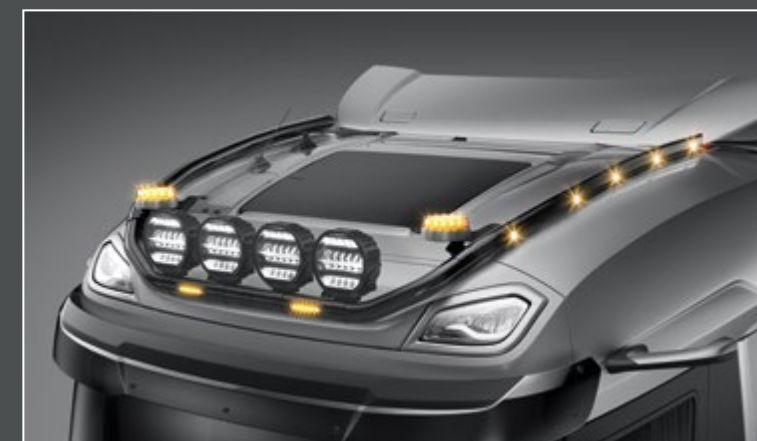
28705-5-B - 28705-11-B - LightFix - SKY-LIGHT "CLASSIC-MAX" DAF XG (28705-5-B) / DAF XF (28705-11-B) Lightbar for mounting a maximum of 4 spotlights and 2 beacons stainless steel - black powdercoated - Ø 70mm - prewired incl. 8 amber LED on the side and red LED in the tube ends
