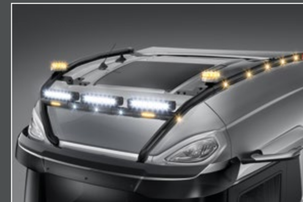
28706-9-B - LightFix - SKY-LIGHT "H-MAX" Lightbar for mounting a maximum of 6 spotlights and 2 beacons stainless steel - black powdercoated - Ø 70mm - prewired incl. 8 amber LED on the side and red LED in the tube ends
