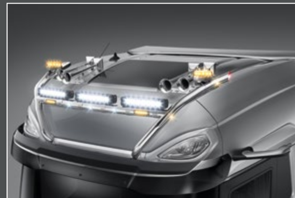
28706-8-P - LightFix - SKY-LIGHT "H-TYPE" Lightbar for mounting a maximum of 6 spotlights and 2 beacons stainless steel - polished - Ø 70mm - prewired incl. red LED in the tube ends
