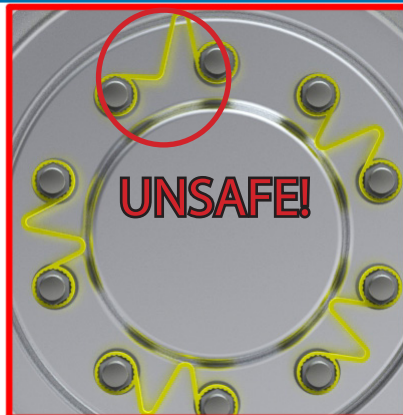
Danger - wheel nuts have loosened!
