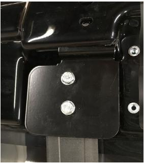
2.3 Mount the hook sleeve #4155 between the washer and sun visor and tighten the screws. With mirror adapter it is not nesessary to use sleeve #4155.
