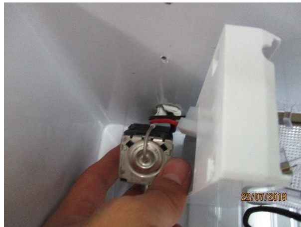
9. Remove the thermostat and reverse the procedure to replace it
