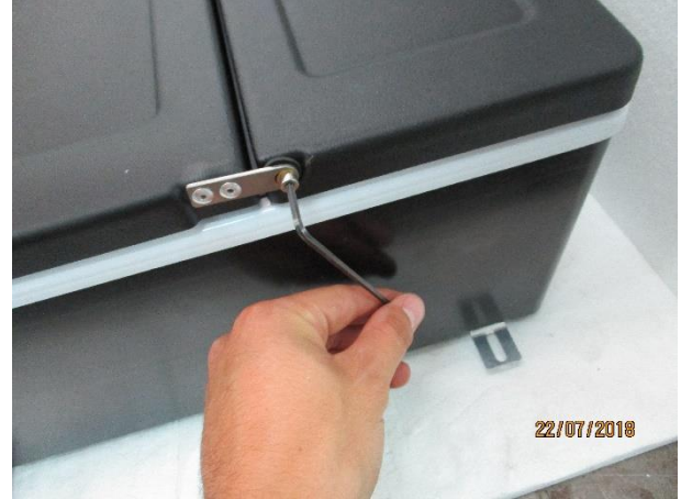
2. Unscrew the protection lid (4 screws)
