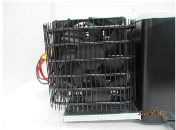
4. Cut the 4 cable ties fixing the fan, disconnect the fan's wire from the ECU and reverse the procedure to replace it
