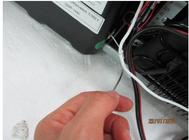
8. Pull the thermostat's bulb
