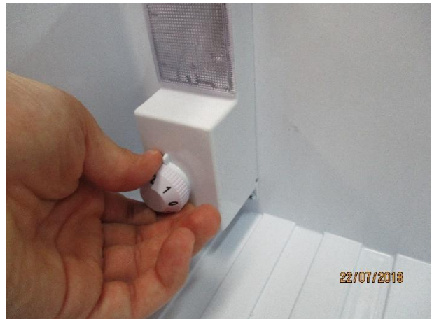
4. Remove the thermostat's knob
