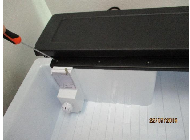
2. Unscrew the protection lid (4 screws)
