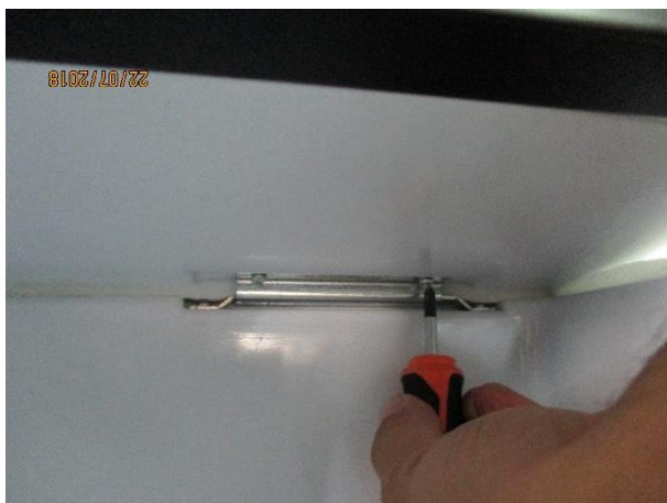
3. Unscrew the hinge fixing the protection lid (2 screws) and remove the lid
