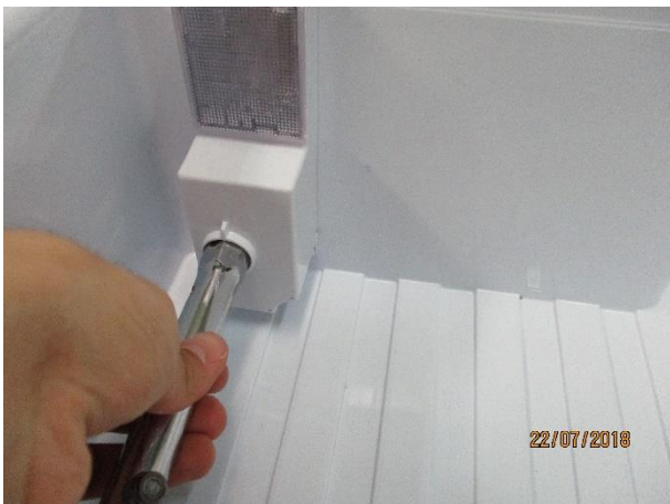
5. Unscrew the screw nut fixing the thermostat
