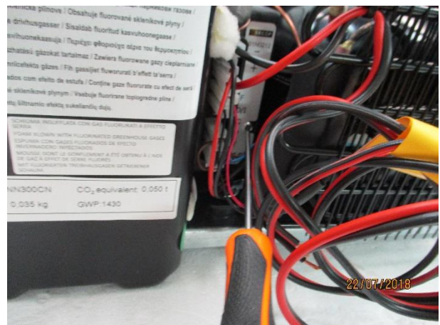
4. Unscrew the bolt fixing the ECU, disconnect the wires and remove it
