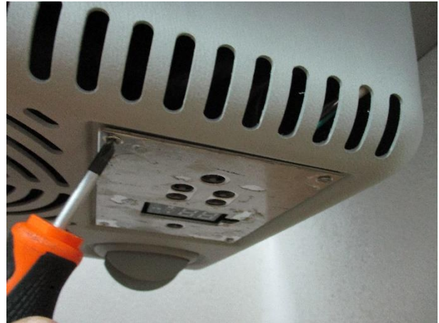
2. Unscrew the bolts fixing the control panel (4 screws)
