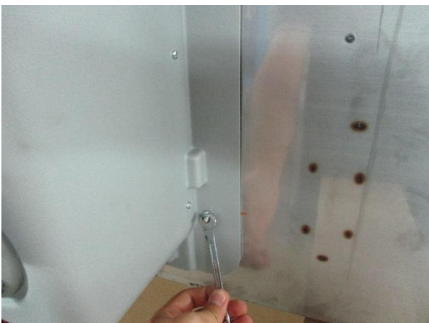
5. Unscrew the 4 screw-nut fixing the air diffuser
