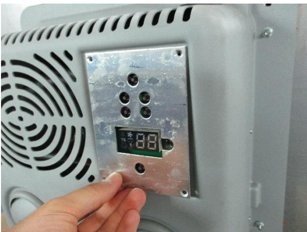
3. Push upward and pull the control panel to remove it
