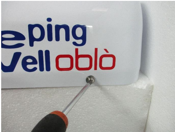
1. Unscrew the bolts fixing the cover and remove it (9 screws)
