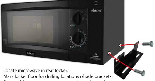
Ensure side brackets are correct height to allow micro- wave door to open once fitted in locker. Drill locker floor and fix brackets to floor with screws supplied.
