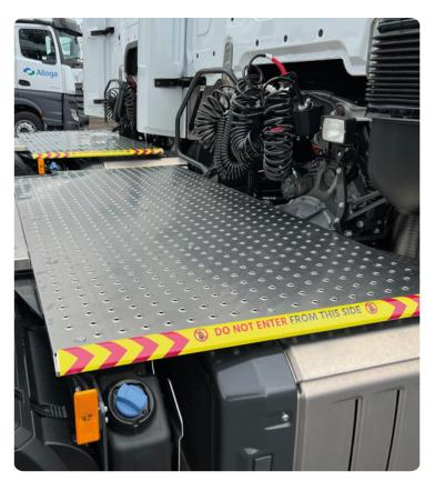
By creating a new sub-frame which raises the catwalk to a level platform, we are able to create a large, safe, anti-slip working area behind the cab.
