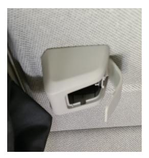
Step 2: Replace the factory metal spacer from the "Step 4" with the supplied "15mm spacer" and the "Scania top bracket 0636";
