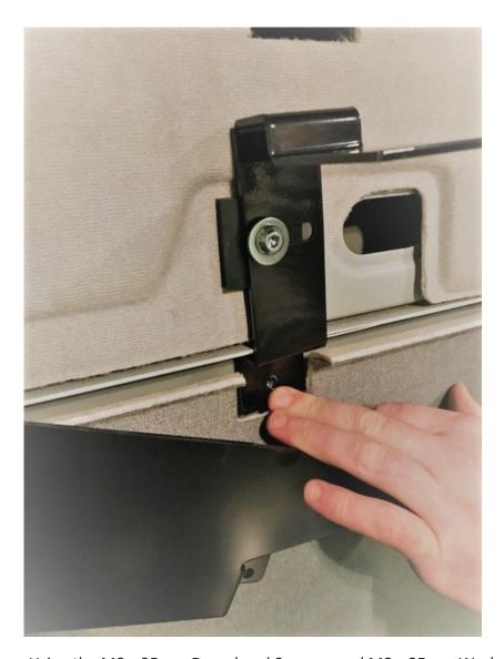
Using the M8 x 25mm Domehead Screws, and M8 x 25mm Washers, Bolt the four brackets onto the back wall, into the Nut Inserts fitted previously.
