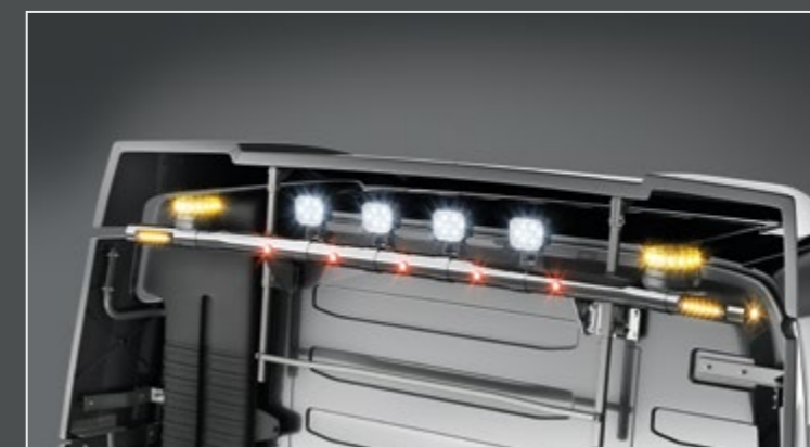
TLG23715-3-P /-B - LightFix - REAR-LIGHT Sleeper Cab / Globetrotter / Globetrotter XL / Globetrotter XXL Lightbar for mounting a maximum of 4 work lamps and 2 beacons Stainless steel - polished or black powdercoated - Ø 70mm - prewired
