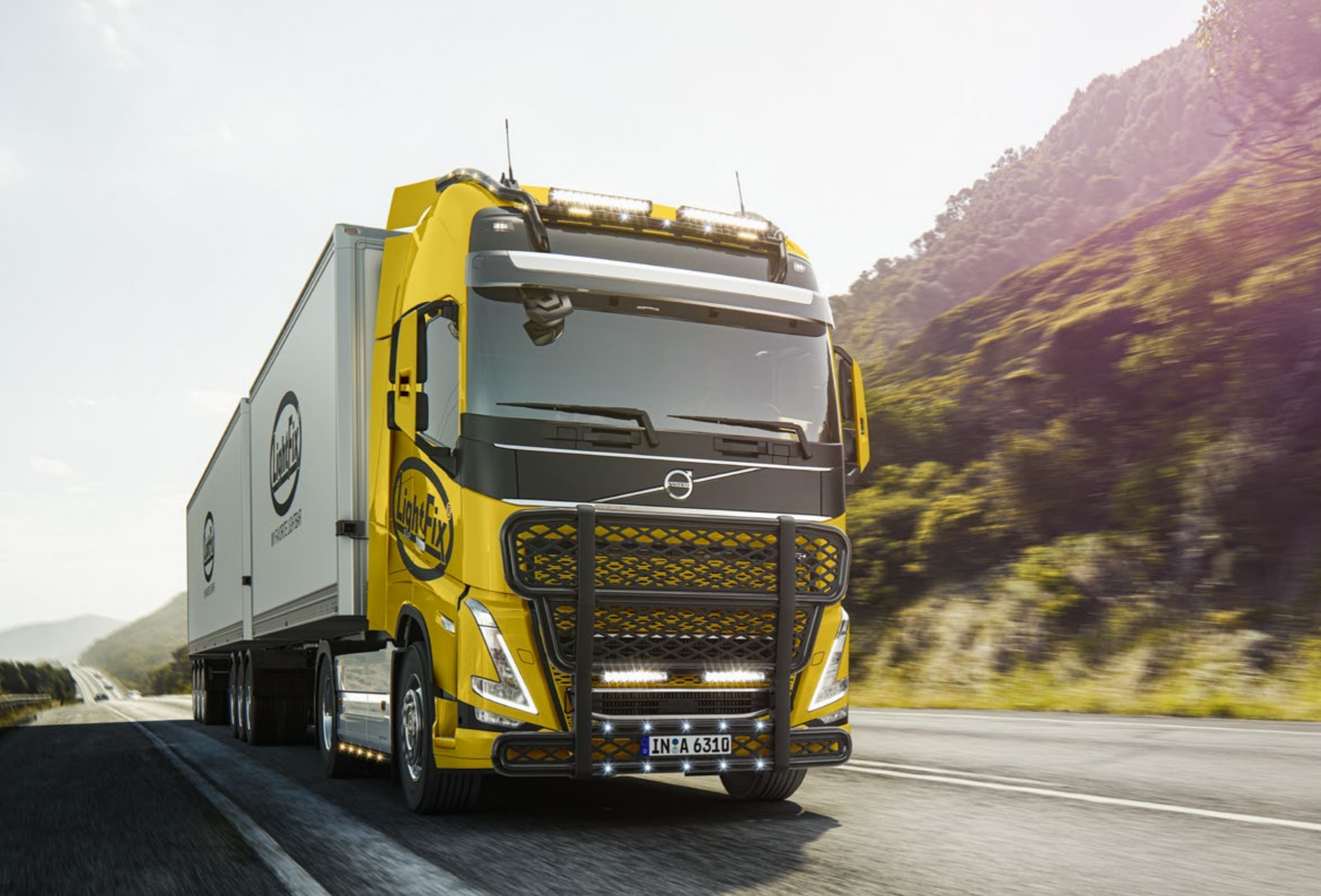
TLG23704-2-B - LightFix - SKY-LIGHT Globetrotter / Globetrotter XL / Globetrotter XXL Lightbar for mounting a maximum of 6 spotlights and 2 beacons Stainless steel - black powdercoated - Ø 70mm - prewired
