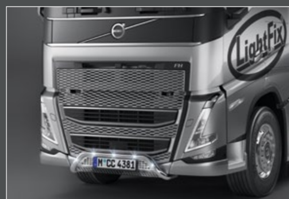
TLG23740-2-P /-B - LightFix - FRONT-LINER "TARGA" Stainless steel LED-lightbar at the front polished or black powdercoated - Ø 60mm - prewired Full LED-set included
