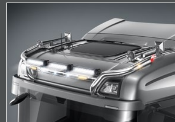
24705-9-P - LightFix - SKY-LIGHT "WILDLIFE" Lightbar for mounting a maximum of 6 spotlights and 2 beacons stainless steel - polished - Ø 70mm - prewired red LEDs in the tube ends
