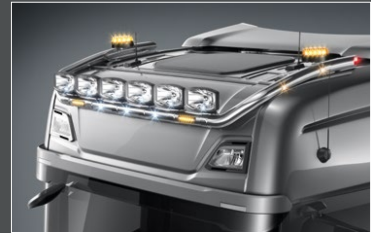
24705-10-P - LightFix - SKY-LIGHT "MAXIMUM" Lightbar for mounting a maximum of 6 spotlights and 2 beacons stainless steel - polished - Ø 70mm - prewired amber LEDs on the side and red LEDs in the tube ends
