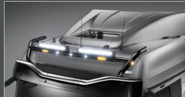
21702-5-B - LightFix - SKY-LIGHT "H-TYPE" Lightbar for mounting a maximum of 6 spotlights and 2 beacons stainless steel - black powdercoated (paintable) - Ø 70mm - prewired red LEDs in the tube ends Note: also suitable for INDIVIDUAL sun visor
