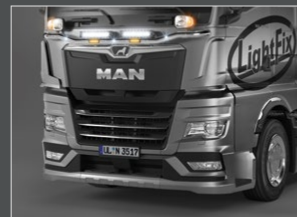
21750-3-P - LightFix - PLOW-LIGHT Lightbar at the front for mounting 2 main headlights and 4 spotlights Stainless steel - polished - Ø 70mm - prewired suitable for snow plows and municipal vehicles
