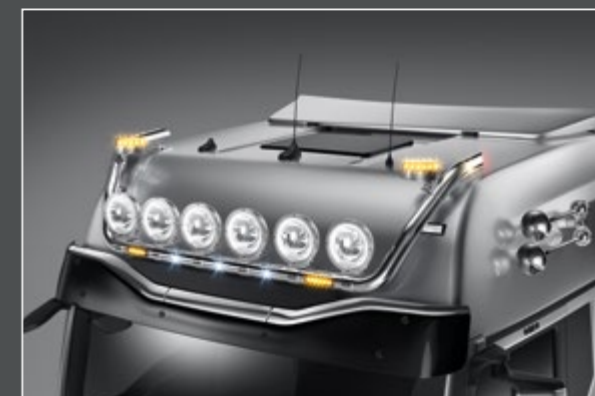
21706-4-P - LightFix - SKY-LIGHT "WILDLIFE" Lightbar for mounting a maximum of 6 spotlights and 2 beacons stainless steel - polished - Ø 70mm - prewired red LEDs in the tube ends Note: for model range until 2021 select 21705-4-P
