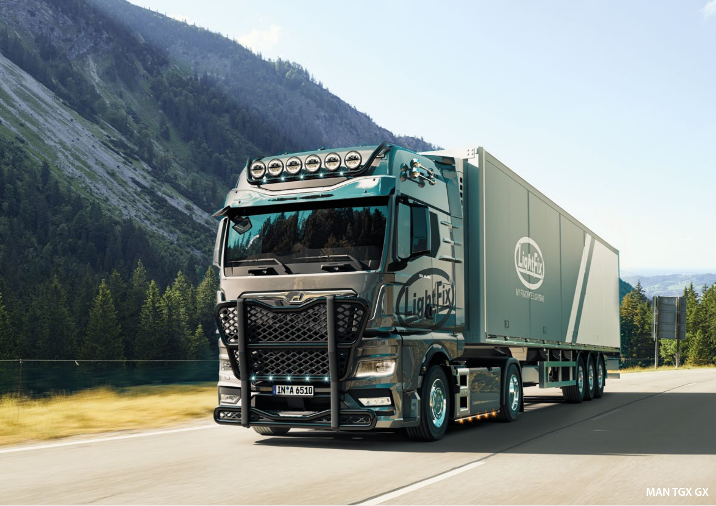
21705-6-B - LightFix - SKY-LIGHT "H-TYPE" Lightbar for mounting a maximum of 6 spotlights and 2 beacons stainless steel - black powdercoated (paintable) - Ø 70mm - prewired red LEDs in the tube ends Note: also suitable for model range until 2021
