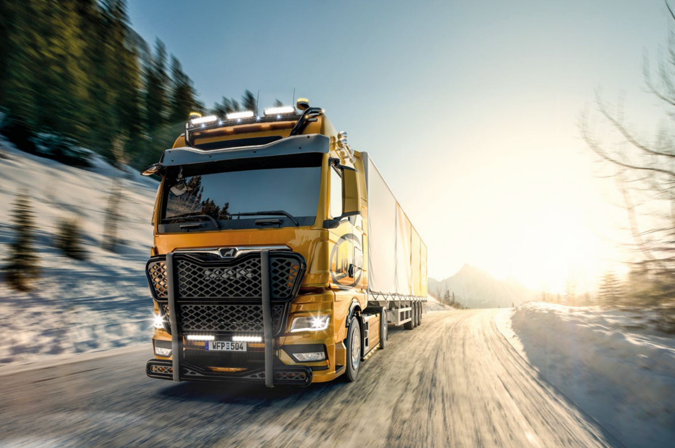
21748-5-B / 21748-6-B - LightFix - CAB-LINER - TGX GX / GM MAN TGX GX (21748-5-B) / MAN TGX GM (21748-6-B) Stainless steel LED-lightbar for driver and passenger side black powdercoated - Ø 70mm - prewired - Full LED-set included
