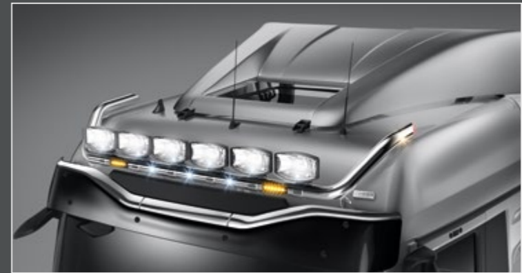
21702-9-P - LightFix - SKY-LIGHT "WILDLIFE" Lightbar for mounting a maximum of 6 spotlights and 2 beacons stainless steel - polished - Ø 70mm - prewired red LEDs in the tube ends Note: for model range until 2021 select 21702-4-P
