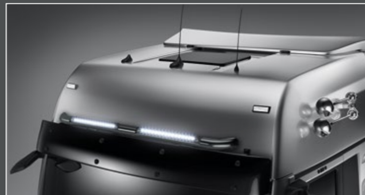
21705-3-B - LightFix - SKY-LIGHT "SLIM" Lightbar for mounting 2 integrated LED spotlights stainless steel - black powdercoated (paintable) - Ø 70mm - prewired Note: not suitable for model range from 2022
