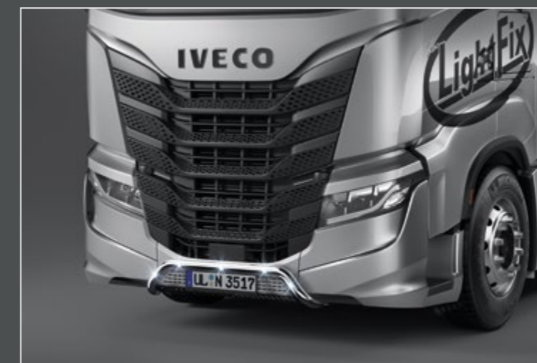
27741-1-P /-B - LightFix - FRONT-LINER "TARGA" Stainless steel LED-lightbar at the front with overrun protection polished or black powdercoated - Ø 60mm - prewired Full LED-set included
