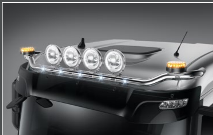
27706-1-P - LightFix - SKY-LIGHT "WING" Lightbar for mounting a maximum of 6 spotlights and 2 beacons stainless steel - polished - Ø 70mm - prewired
