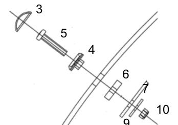
Mount the side brackets with M6x40mm screw use the 6mm rubber washers between side bracket and the acrylic part.
