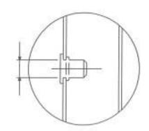
But Sikaflex on the holes and mount the rivet nuts as shown on the drawing.
