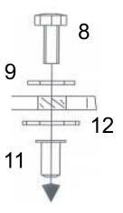
But Sikaflex on the topside of the acrylicpart which toutches the cabin. Mount the acrylicpart on the brackets and tighten all screws.
