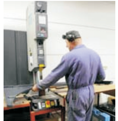
We use the latest CAD / CAM technology in designing the parts and making the tools. We can use clients 3-D designs or we can offer the full service in measuring, designing and producing the tools and parts. Ultrasonic welding is used to attach plastic pieces together.
